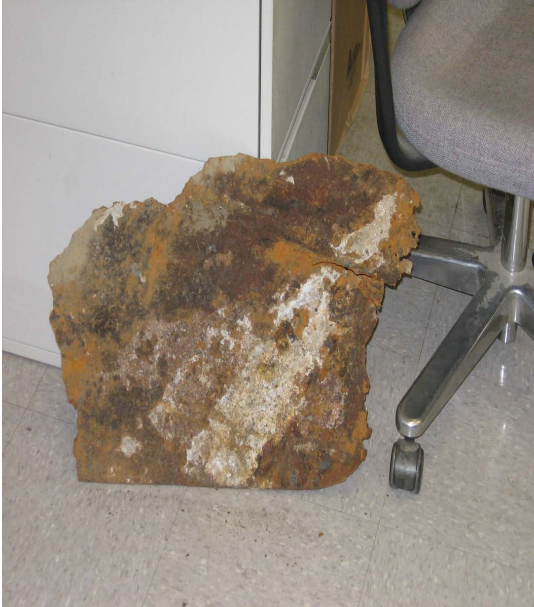
Piece of pump #1 interior
