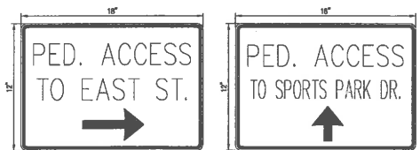
PEDESTRIAN ACCESS DIRECTIONAL SIGNS NTS
