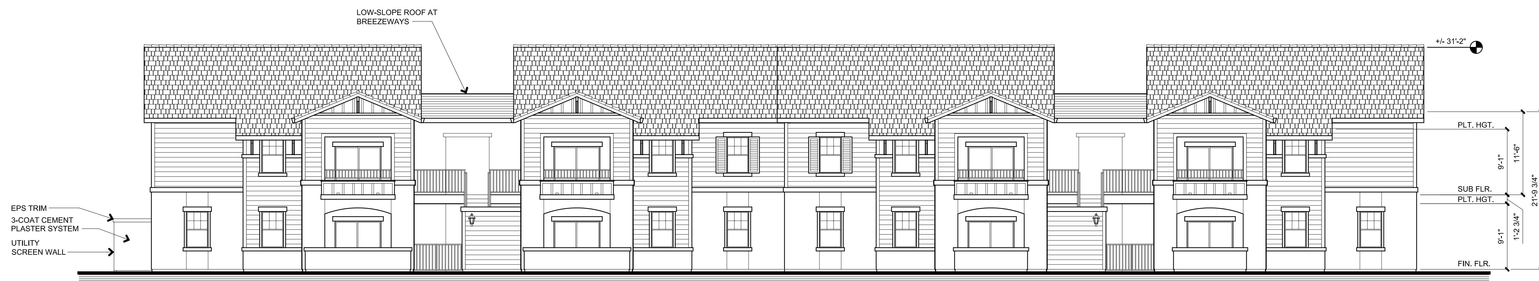
BUILDING H (TYPE 4) - NORTH ELEVATION
