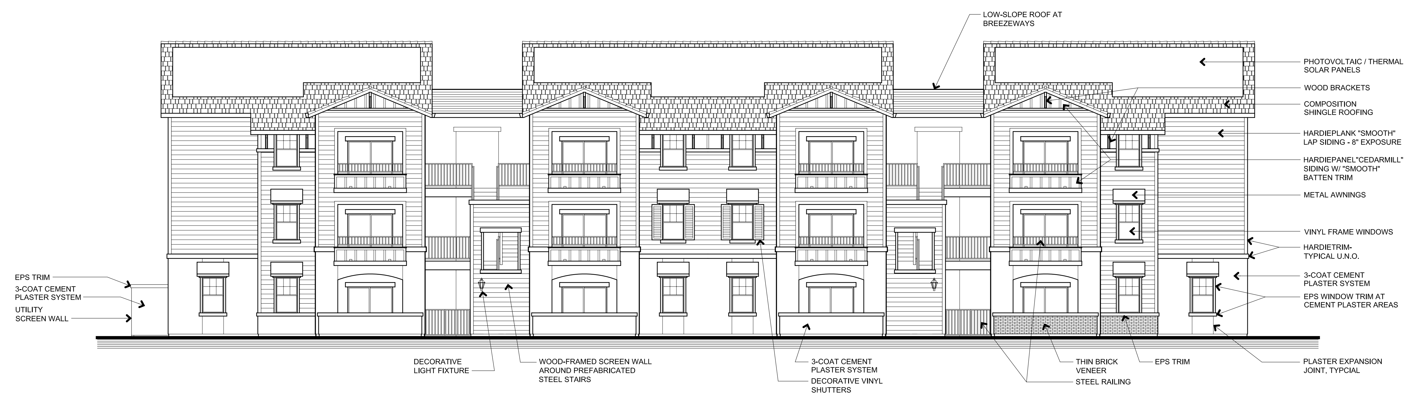
BUILDING B (TYPE 2) - SOUTH ELEVATION
