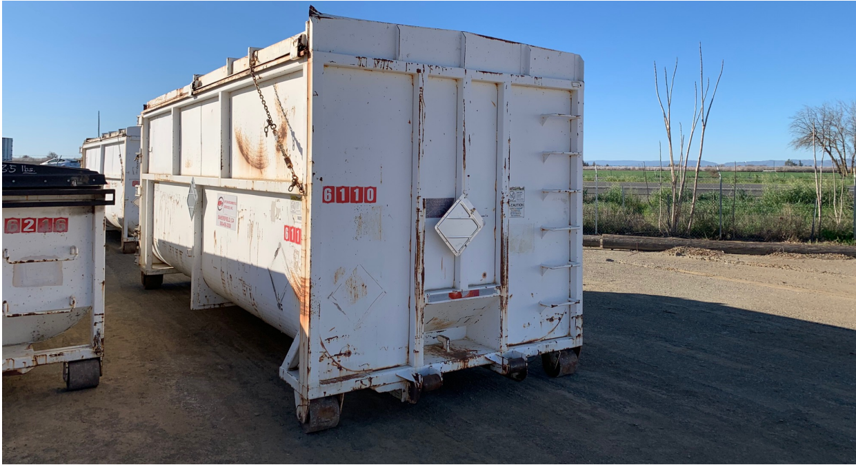
Tall covered roll-off bin for construction materials, debris and non-hazardous soils
