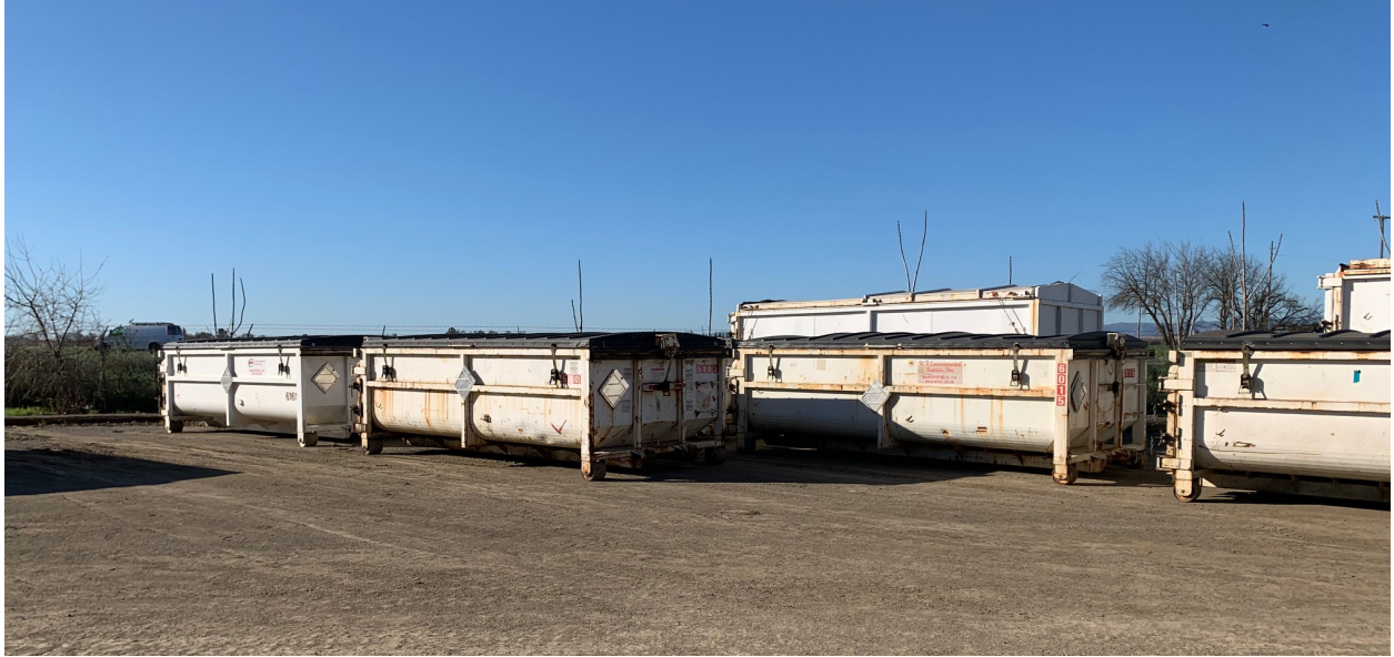
Covered roll-off bins for construction materials, debris and non-hazardous soils
