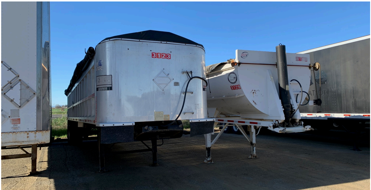
Open, tarp-covered trailers for non-hazardous demolition debris
