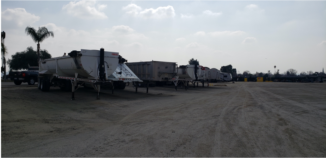
Open, tarp-covered trailers for non-hazardous demolition debris
