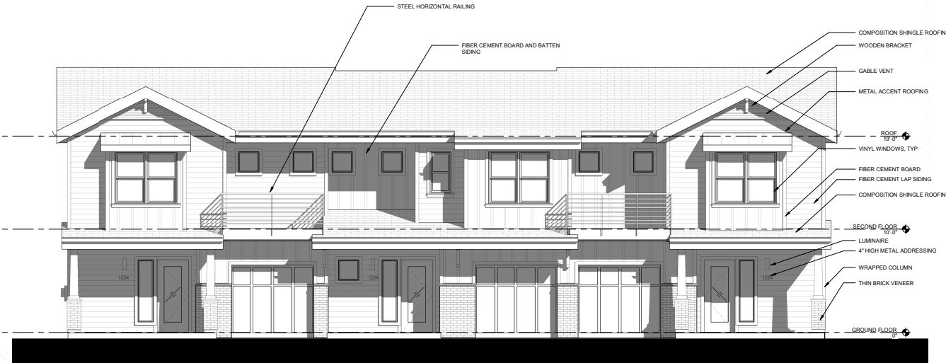
① FRONT ELEVATION - DRIVE AISLE ENTRY 1/4" = 1'-0"
