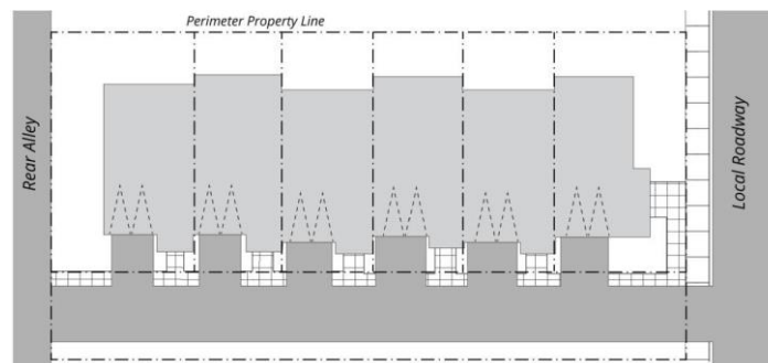
FIGURE 17.56.040.E-4: ATTACHED UNITS WITH TUCK-UNDER GARAGES (EXAMPLE CONFIGURATION)
