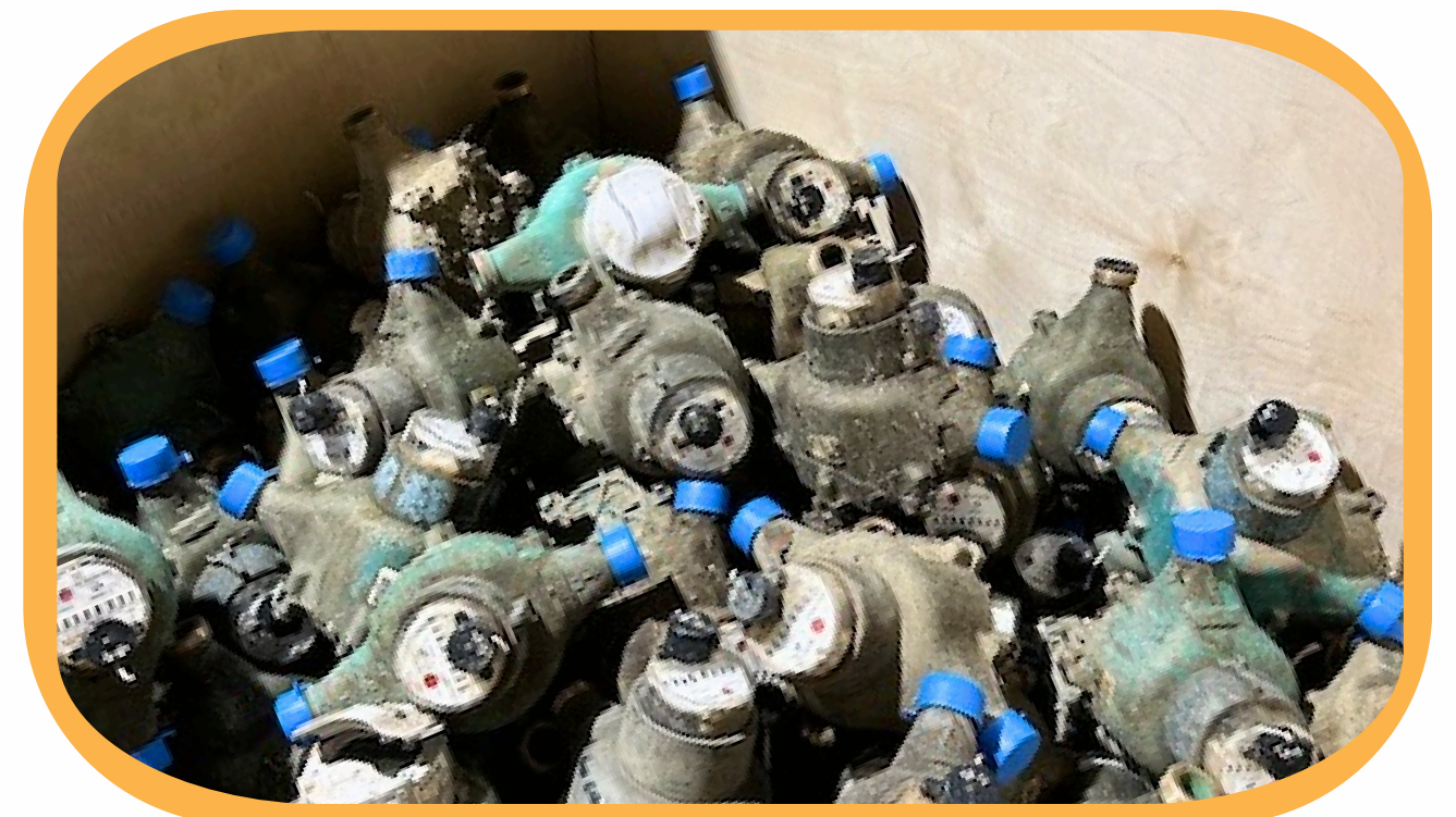
Older water meter units removed as part of the Water Department's ongoing meter replacement project.
